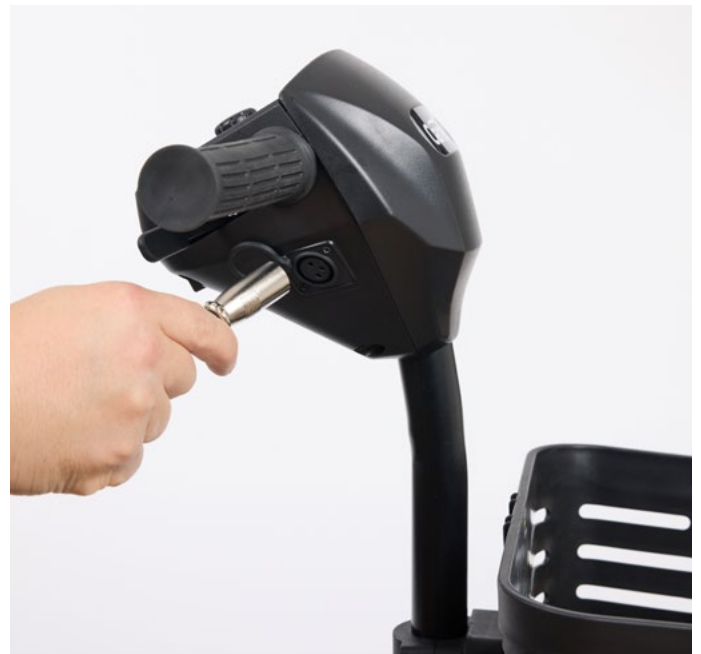
8. Charge the scooter for 12-16 hours before first use.
