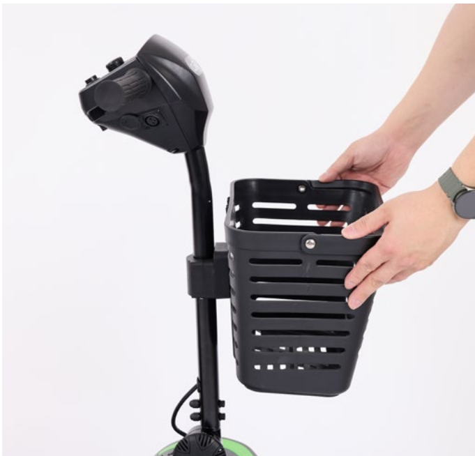
7. Place the basket onto the basket hooks.
