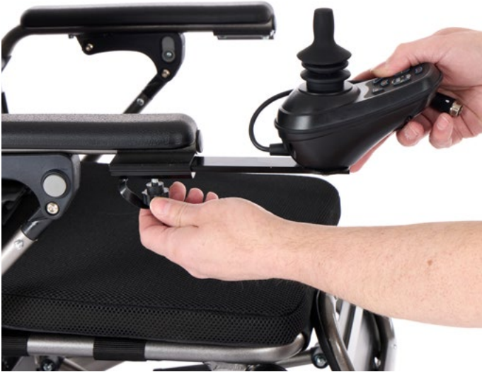
5. Insert the joystick assembly into the bracket on the underside of the armrest, then secure using the bolt provided.
