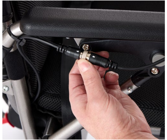
6. Connect the joystick cables together.
