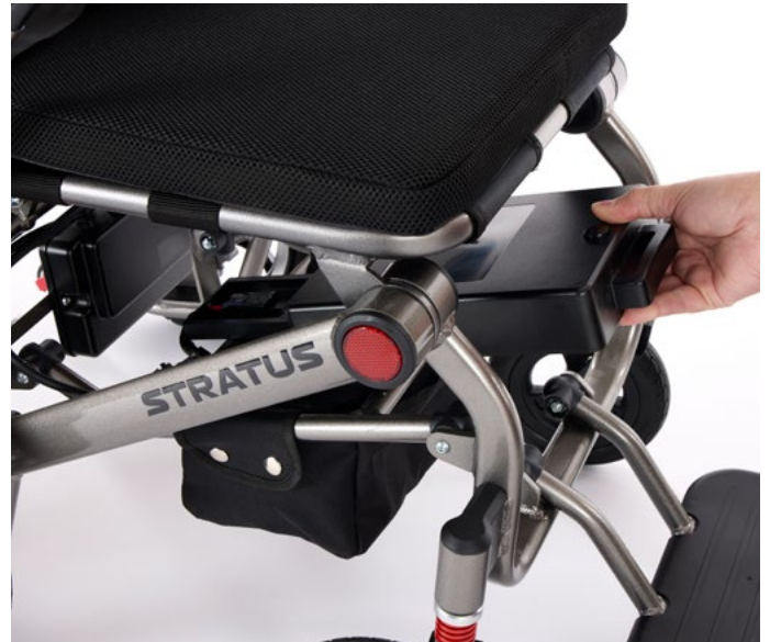
8. Insert the battery into the battery slot.
