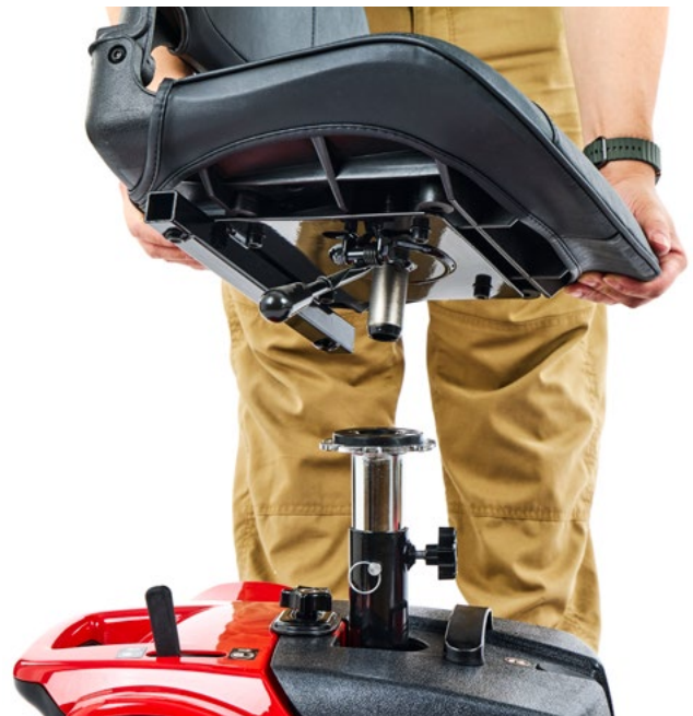
8. Lower the seat onto the seat post.
