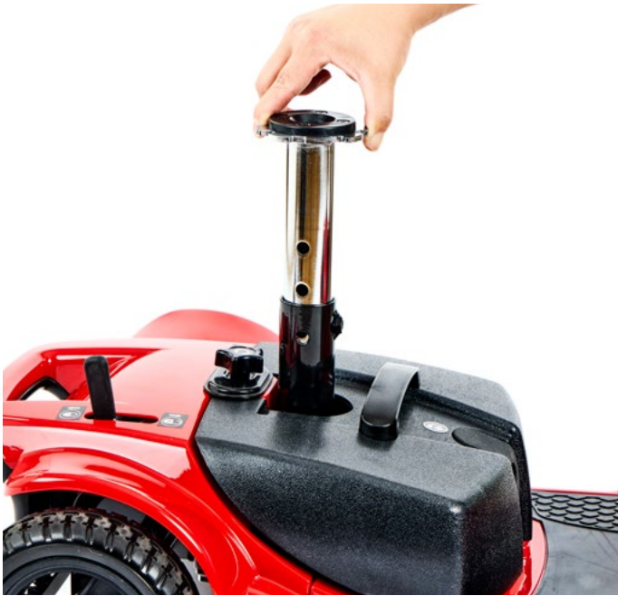
5. Insert the seat post into the scooter base.
