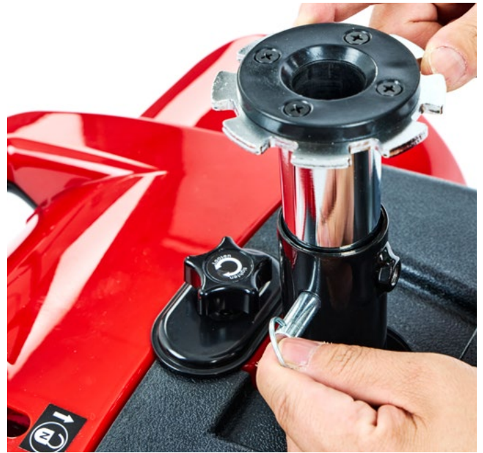
6. Insert the seat post pin to secure the seat post height.
