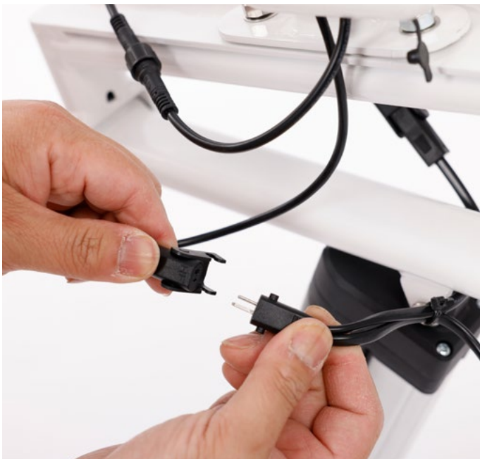
7. Connect the battery and actuator plugs together.
