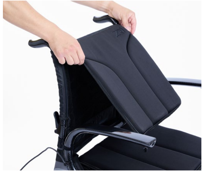
6. Place the backrest cushion onto the back of the powerchair.
