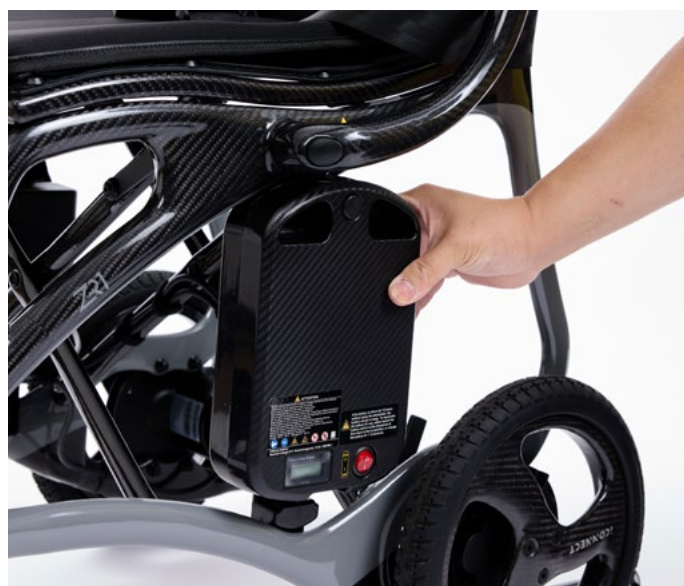
12. Insert the battery into the side frame holder.
