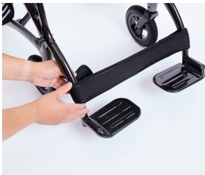
11. Secure the calf strap to the powerchair using the velcro.
