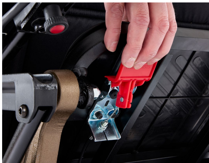
2. Lift and hold the red seat lever.
