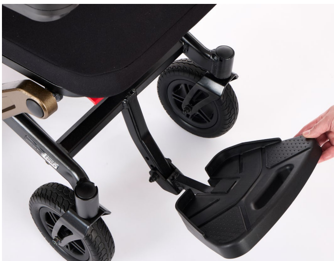
1. Fold the footplate upwards.
