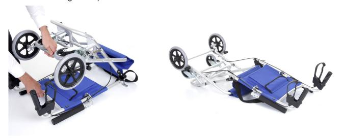
3. Place all four wheels on the floor and push the Seat folding tube up towards the seat of the chair. The folding brackets on either side should click horizontally into place.
