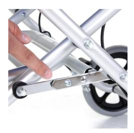
4. Ensure the Backrest Folding locks are pointing away from the chair and raise the backrest into position, pull the material strap up to detract the locking pins and continue to raise the backrest up until the locking pins will insert into the frame, release the material strap to lock in place.
