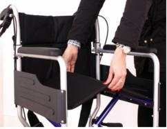
The backrest also has a half-folding back which can be used to make the Traveller even more compact. Push the black paddle at the rear of the chair with your thumb whilst pulling the handle down.
