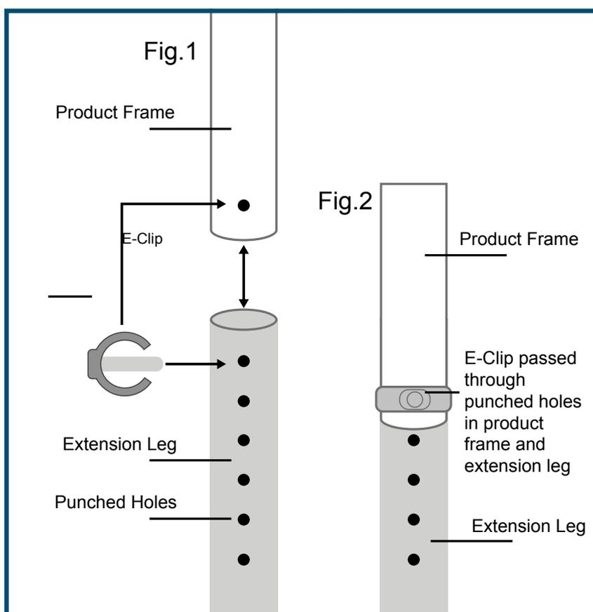
Check that the trolley is sitting evenly on the floor and there is no excessive rocking or the trolley is tilting to one side. If this is the case, please do not use the trolley, but repeat the above steps to correct the problem or contact your supplier for service support.
