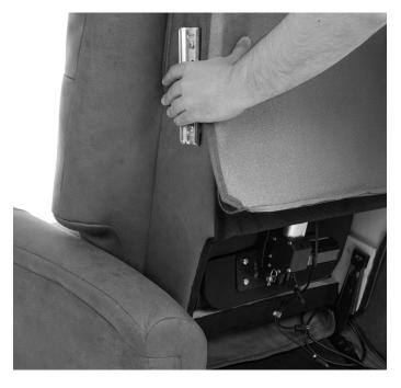
5. Lower the backrest onto the seat base prongs, then firmly push downwards.
