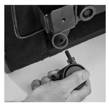
2. Tilt the base of the chair forwards, then insert the locking castors into the rear of the mechanism.
