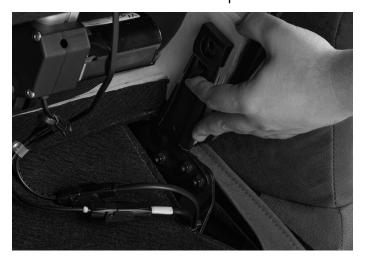
3. Release the locking clips on either side of the backrest whilst pulling the backrest upwards.
