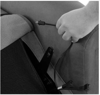
4. Lift the power cable away from the seat base prong and place to one side.
