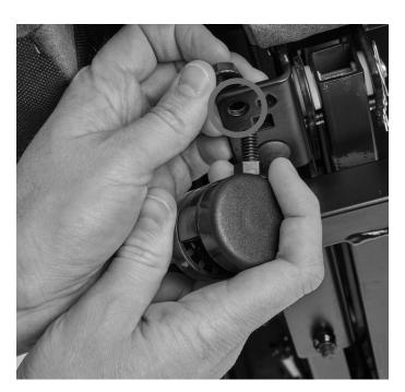
3. Tilt the base of the chair backwards, then insert the castors into the front of the mechanism.
