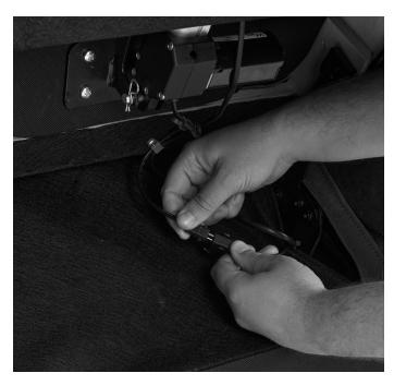
7. Lift the backrest flap to reveal the chairs wiring, then connect the power cables together.
