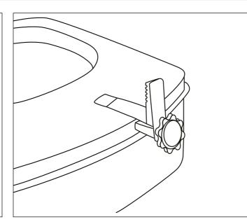
2. Insert the hand screw assembly into the base of the raised toilet seat, then repeat on the other side.
