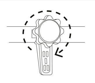
4. Tighten the hand screws to secure the raised toilet seat to the toilet bowl.
