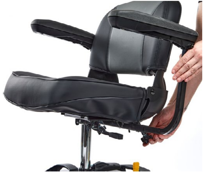
6. Insert the armrest(s) into the lower seat bracket(s) and secure using the armrest bolt(s).
