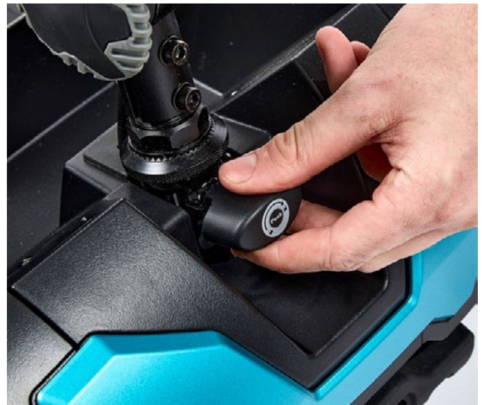
8. Push the tiller locking mechanism inwards, then twist anticlockwise to unlock the tiller.
