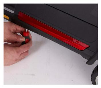
1. Using a Pozi screwdriver, unscrew the side shrouds from the scooter body, then lift them away from the scooter.
