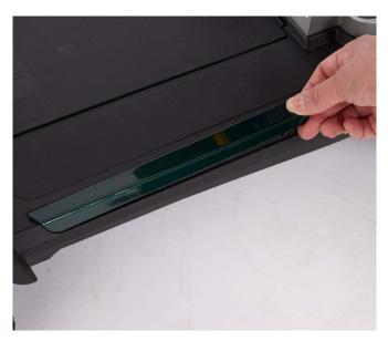
2. Place the new shrouds into position, then secure them in place using a Pozi screwdriver.
