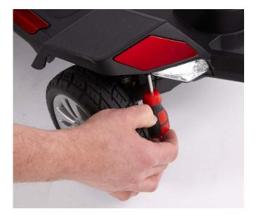
1. Using a Pozi screwdriver, unscrew the front shrouds from the scooter body, then lift them away from the scooter.
