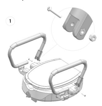
Insert the nut and bolt into the armrest as indicated above, be careful not to over-tighten.
